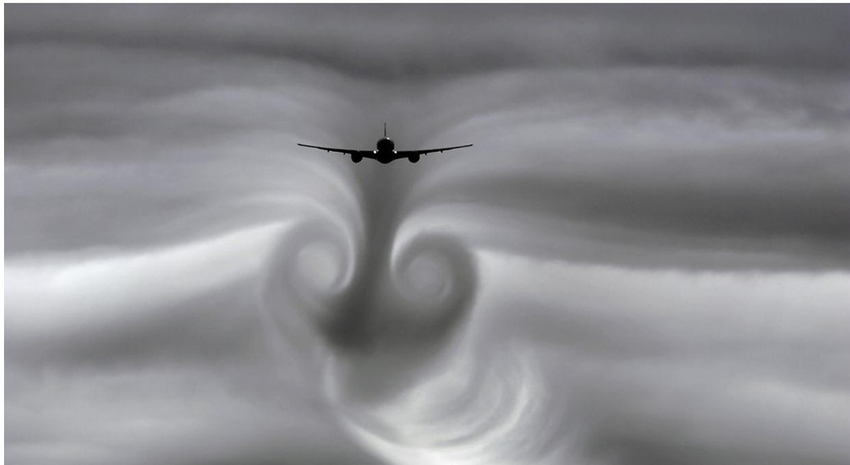
Figure 1: *Wingtip vortex and downwash of an airplane flying in the clouds*
