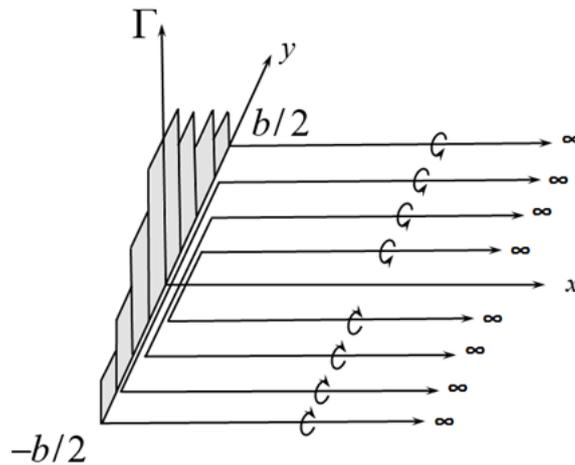
Figure 5: Illustration of multiple horseshoe vortices at the trailing edge of the wing, together with the circulation distribution
