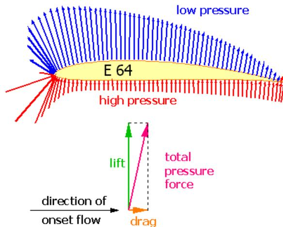
Figure 2: Pressure distribution on wing section [2]
