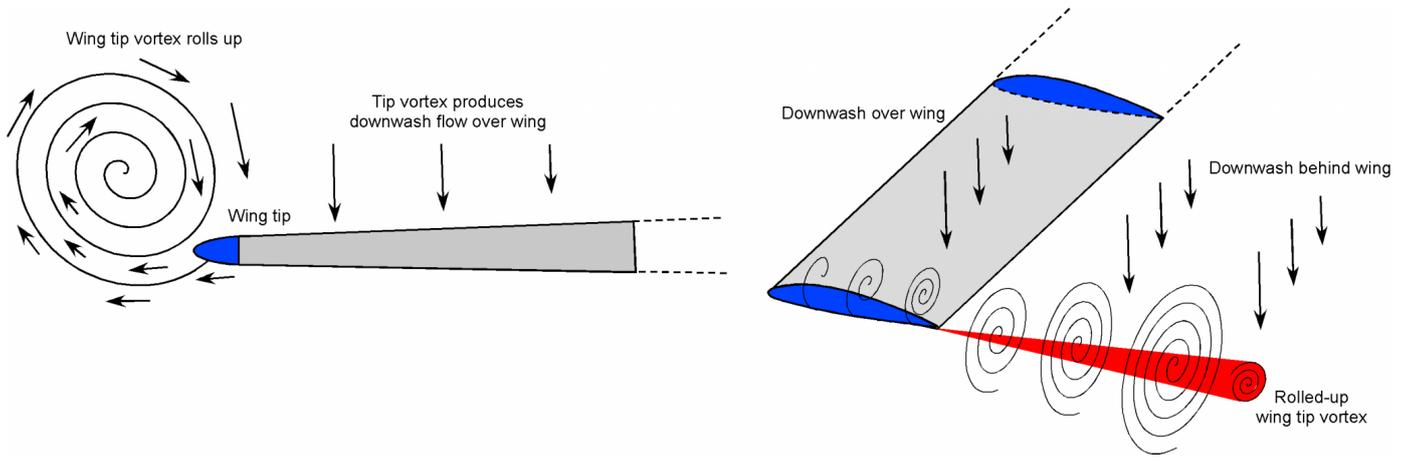
Figure 3: *Wing vortex and down-wash on a wing [3]*
