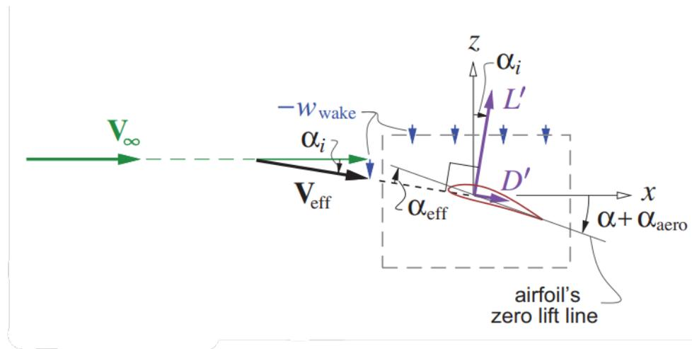
Figure 4: *Forces on finite wing with wake, showing induced drag [4]*
