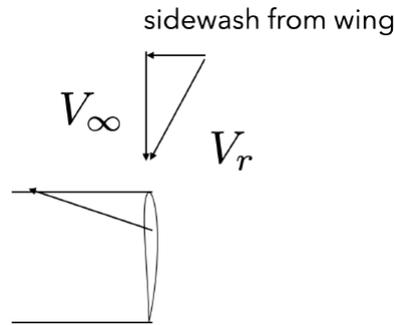
Figure 8: Sidewash induced by the wing onto the winglet and the lift direction [9]
