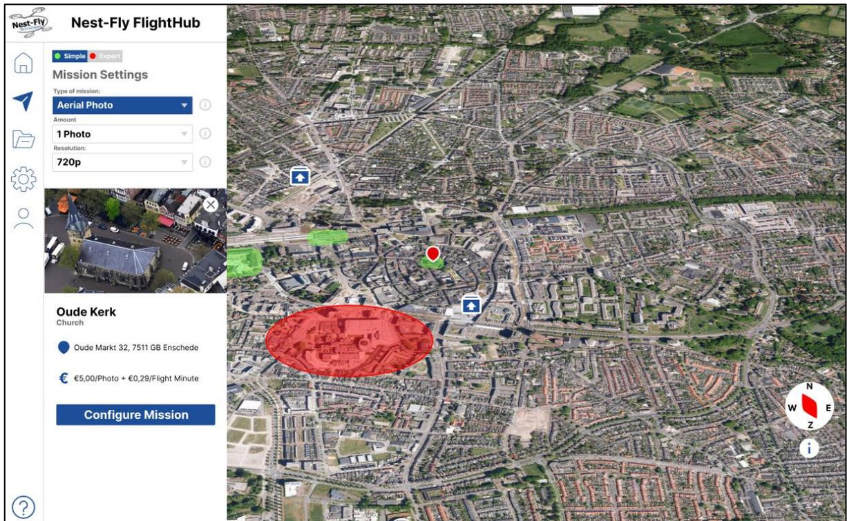
Figure 6.14 Drone Mission-planning interface when a building has been selected
