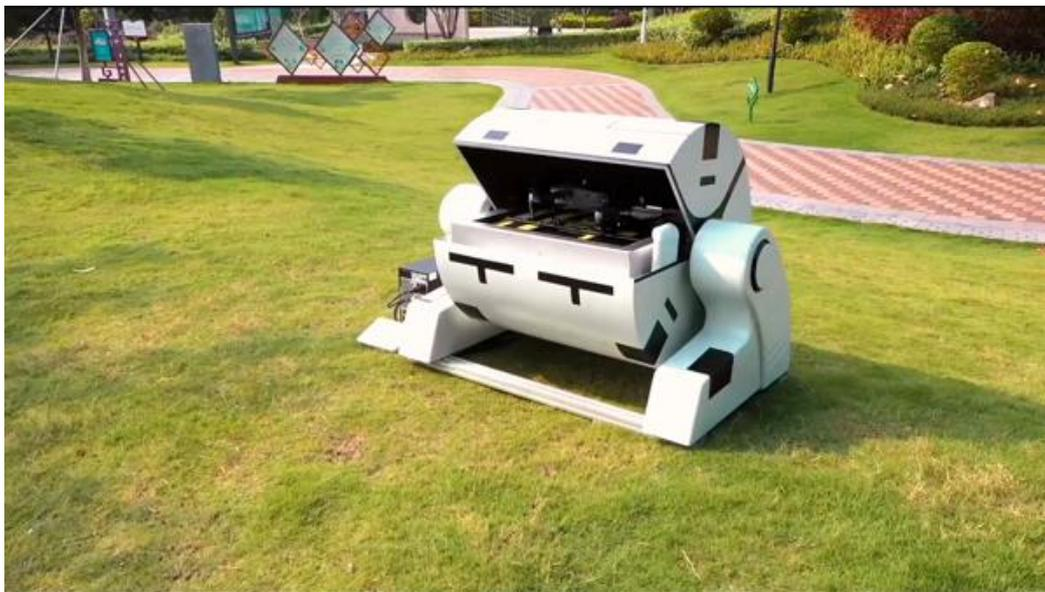
Figure 2.9 Drone Docking System of Heisha [41]
