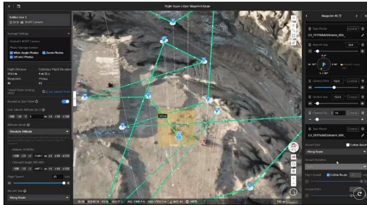
Figure 2.4 DJI FlightHub 2, an interface for the DJI Dock Drone Docking System [36]
