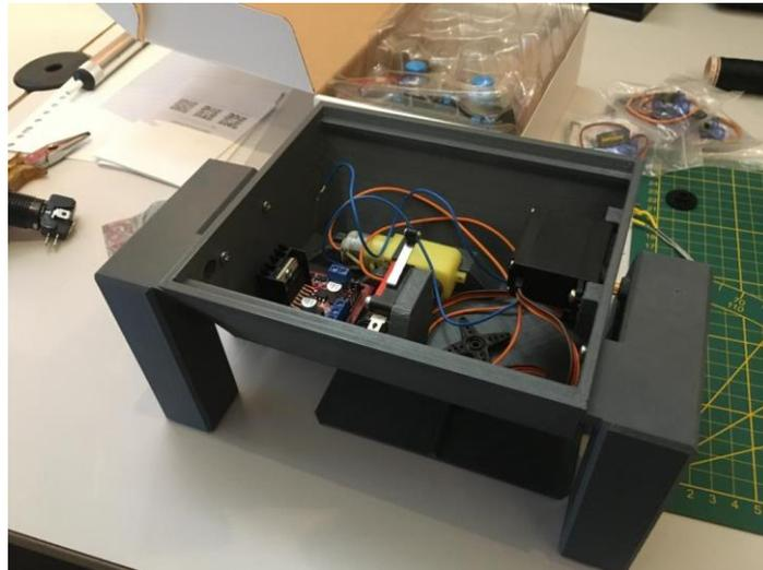
*Figure 12.6 Electronics inside the Drone Docking System*
