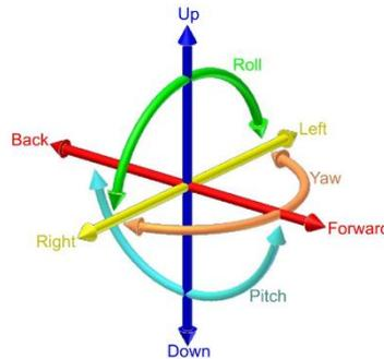
*Figure 2.2 Translations and rotations of a Drone in 3D space [25]*
